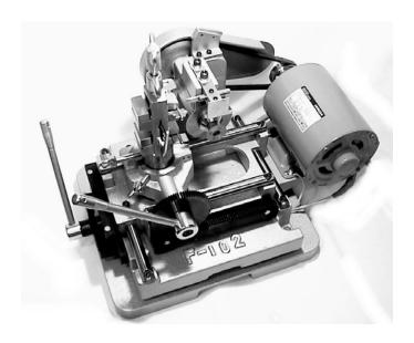
This machine is designed to duplicate safe deposit keys, warded padlock keys, and bit type keys. Through the use of two cutters and extremely versatile key vises, keys can receive cuts on different edges without being removed from the vise.
