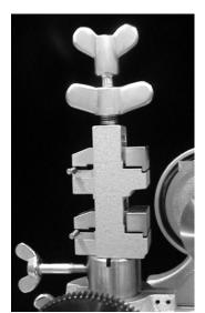
The entire vise assembly can be rotated to various positions and locked in place. One side of each jaw is designed for flat steel keys; the opposite side is for bit keys.
