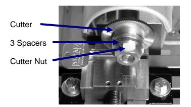
**KEY VISE:** Position the key as shown in the illustration, and secure it by tightening the vise. To reposition the key vise, loosen the hex bolts that secure it to the milling table. It can be repositioned along any of the tracks on the table.
