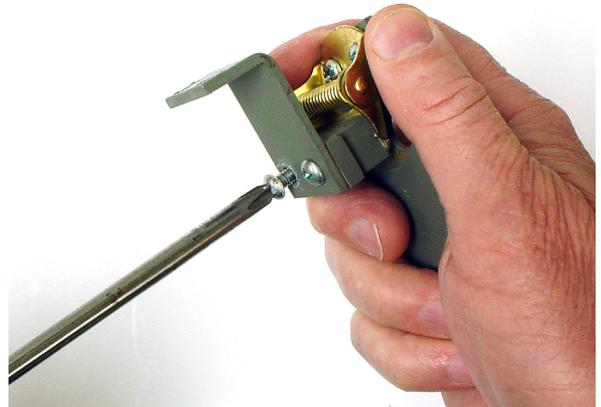
Step 3: Using an 11/32" nut driver or wrench, remove the hinge nuts from the long, flat handle bracket. Once these are out, remove the two 8-32 screws from the opposite side of the hinge. Now the old hinge (with hinge block still attached) can be separated from the handle bracket. These screws and nuts will be re-used, so it's a good idea to wire brush the threads to clean out any dried threadlocker.
