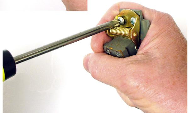
Step 4: Inspect the long handle bracket to make sure it is straight and flat. Sometimes these brackets are bent as a crude form of installation adjustment. This is not recommended. The handle bracket must be flat and straight to work with the 2740-117 retrofit kit. Flatten and/or straighten as necessary.
