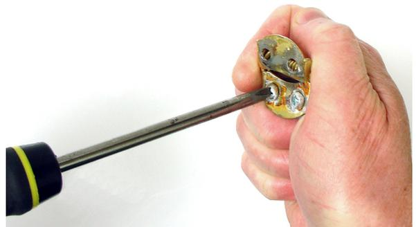
Step 6: Install the new hinge found in the retrofit kit to the steel hinge block. It doesn't make any difference which leaf of the spring is attached to the block. However, the screw holes in the hinge block are slightly offset. Orient the spring with the block's screw holes oriented as shown at right. Use the screws you removed in step 5.
