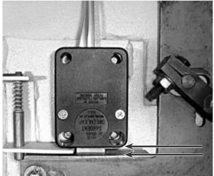
This photo shows a gap between the end of the lock body and the blocking bar of the safe's boltwork (see arrows). This gap should always be a minimum of .150" (3,8 mm).
