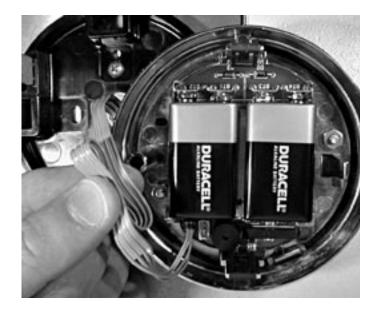
Place the keypad over the base. Make sure the wire cable is still clear of the three spring clips, then push the keypad firmly onto the base. It should snap into place.
