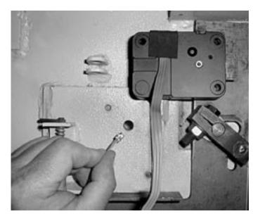
Once you've made sure the wire cable is not crimped or in contact with any sharp surface, attach the lock to the safe's mounting plate. Use the three 1/4-20 (or metric M6) screws provided. Tighten securely so the lock is attached firmly to the plate.
