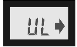
Whenever the Supervisory Combination is redialed, the lock will display **LU (Locked Up)**, and the Subordinate Combination will no longer open the lock.
