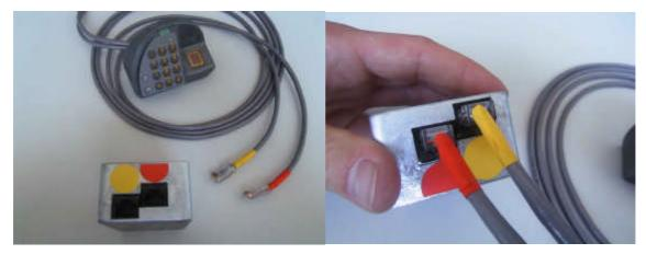
Insert the jack plug, linked either to the external power supply or to the battery box into the lock housing (admitted tension 5-12V, a higher tension damages the lock)
