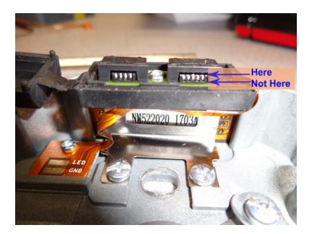
This picture shows the correct position to install the cables into the new style ZIF connectors. One way to check your installation is to give a gentle tug on each of the cables after closing the ZIF connectors. If a cable was slid under, rather than into, a ZIF connector, it will not be locked in place and will slide out again with a little tug.
