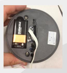
Step 2: The back of the EntryPad will reveal a 9 volt battery. Remove the battery from its compartment.
