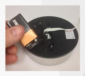
Step 3: Remove the terminal block from the battery.
