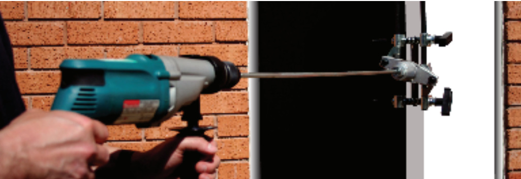
Long Drill Adapter installed on housing
