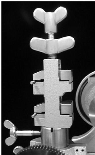
The entire vise assembly can be rotated to various positions and locked in place. One side of each jaw is designed for flat steel keys; the opposite side is for bit keys.
