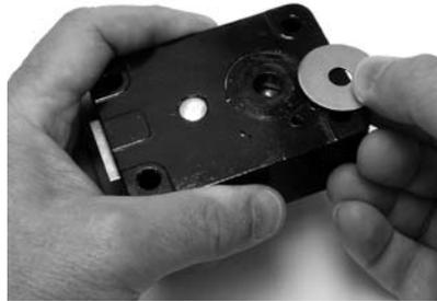
2. Mount the lock in place with four 1/4-20 attaching screws (provided).
