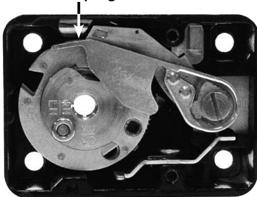
Accelerator Spring in Loaded Position
