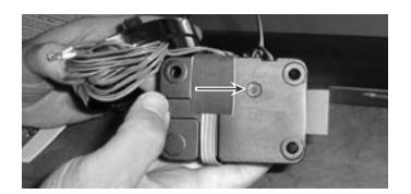
Use a reamer or round file to remove any sharp edges from the wire channel (spindle hole) that might damage the wire cable.
