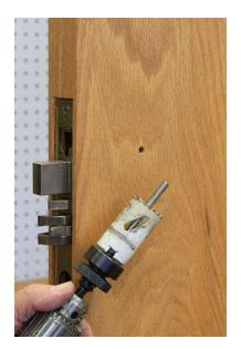
Replace the pilot bit of your hole saw with the supplied drill blank.
