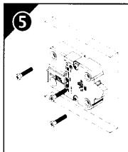
Mount lock with the (3) three US 1/4"-20 mounting screws from the hardware pack (or use M6 screws).
