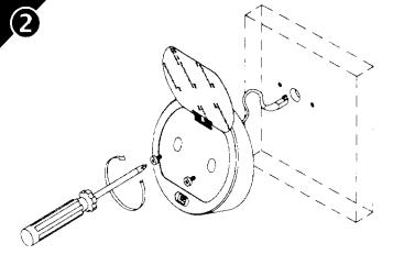
Lift keypad to position shown to expose the mounting holes. Install the 2, 8-32 screws to mount the Entry to the door. Make sure the battery cable is routed through the opening at the bottom of the housing and be careful that the wires are not pinched under the housing.
