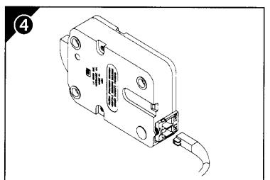
Press the lock's snap connector toward the bottom of the lock. Carefully insert the Entry Cable Plug at the 'ENT' position as shown. Note: Securely fasten the remaining cable down to avoid damage to the cable by moving parts.
