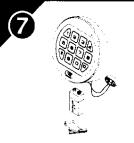
Connect a 9-Volt Alkaline Battery to the battery clip. Insert the battery into the bottom of the entry housing. Install the battery cover in place by placing one side of the cover in position and then pressing the other side into position with your finger.
